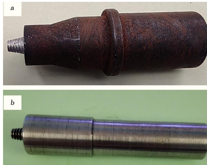
Fig. 1. Images of FSW tool: a —DS-FSW, b —SS-FSW.
